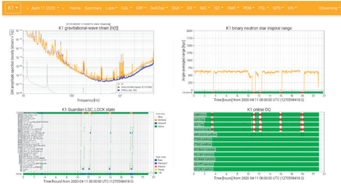
Fig. 4. Example of the KAGRA SummaryPages, used to monitor the interferometer status by on-site team members and for daily checks from remote sites.
